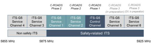
Figure 1 – Current use of the ITS band for infrastructure use cases of C-ROADS [5]. Note that the spectrum is used with listen-before-talk, so that no exclusive allocation is necessary.
